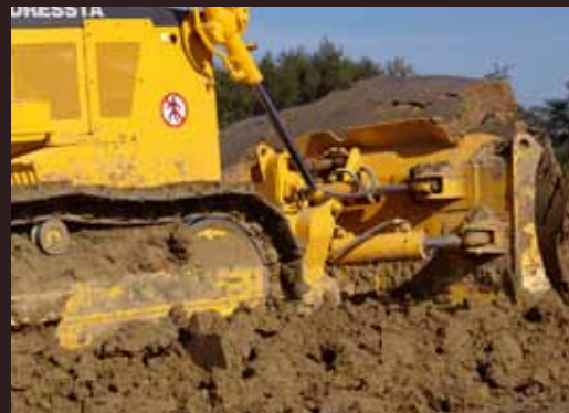
6-way hydraulic angle blade of 3.2 m 3 (4.2 yd 3 ) (STD & LT) and 3.8 m 3 (5.0 yd 3 ) (LGP)
